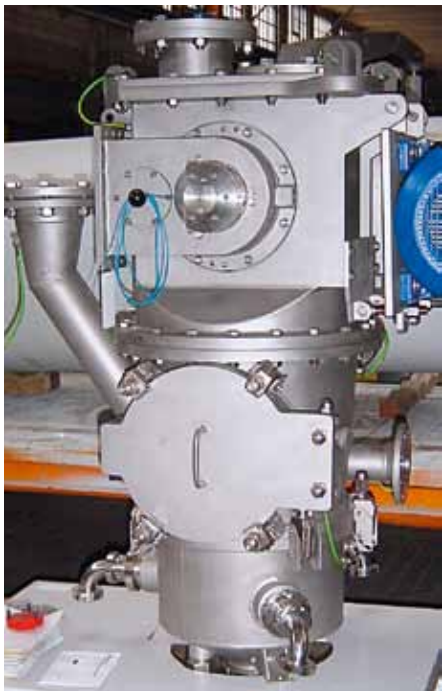
200/400 TTG WITH TURBO TWIN CLASSIFIER HEAD
